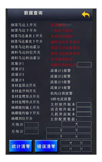
Data query can query the switch status and the position of the pot body, etc. The red light on the upper switch means that the pot body has reached the cooking position and cannot move upwards; in the same way, the red light on the switch can no longer move downwards. It can also detect the working status, software version, hardware version and some other indication status of the flow meter. When everything is normal, you can enter other modes to operate the machine.
